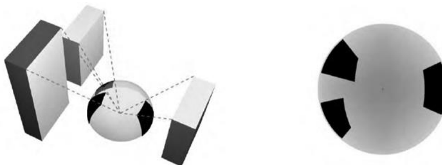
Figure 1.10: Sky View Factor means the extent of sky observed above a point as a proportion of the total possible sky hemisphere above the point.
